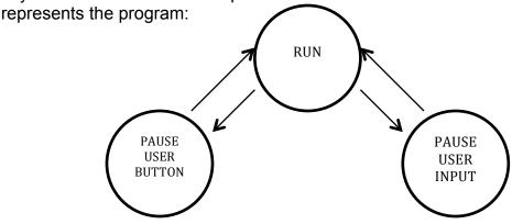
From the *Run* state we can move to the *PauseUserButton* state if the button is pressed. From the *Run* state we can move to the *PauseUserInput* state if the user types a 'p'. We can only exit the *PauseUserButton* to the *Run* state if the user releases the button. Likewise, we can only exit the *PauseUserInput* state if the user types a character 'r'. Note that all the state machine is wrapped around a while(1) and implemented as a switch statement.
